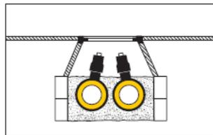
Example of pre-insulated valves buried directly in the ground with access from street level.
