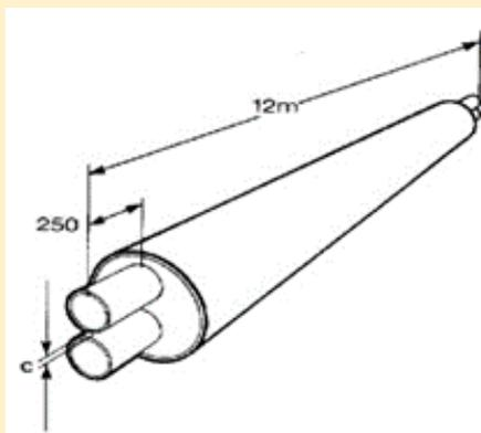
The twin pipe system means that two carrier pipes are placed in one casing pipe with polyurethane foam insulation. The two carrier pipes are fixed together with fix plates and move as a whole. All pipe section ends are provided with fix plates designed for temperature variations between the two carrier pipes of typically maximum 90 °C.
