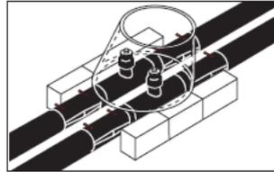
This ensures the free expansion of the pipes and the spindle tops are kept free of sand.
