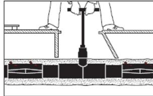
The method shown can also be used for major dimensions, provided that the spindles are tilted to enable operation from the chamber opening.
